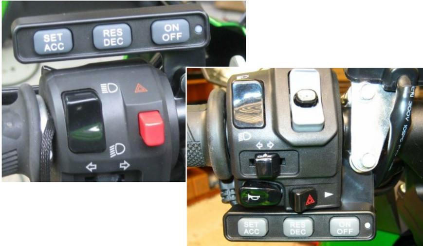
The Motorcycle Electronic Cruise Control is similar in principle to a car cruise control.
