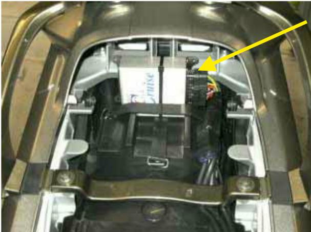
The **Computer (1)** mounts under the rear of the passenger seat.
