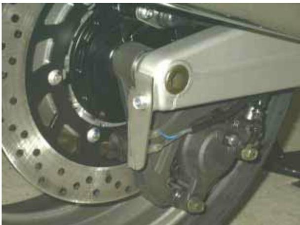
The **Speed sensor (5)** is mounted on the end of the right hand side of the swing arm under the axle pinch bolt. Nickel plated magnets are placed in the heads of the bolts that mount the brake disc.
