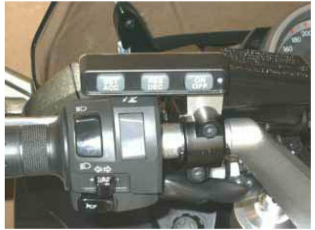
If a tank bag is not normally used on the bike the **Control Switch (7)** may be mounted below the handlebar. This requires a different switch bracket and material must be filed from the lower face of the clutch lever clamp to allow for the thickness of the bracket.
