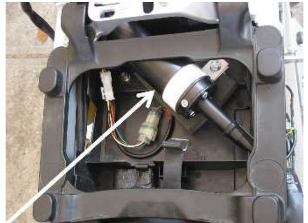
The **Electric Throttle Servo (2)** is bolted inside the storage compartment under the rider's seat. It does not impact on the seat height adjustment Mechanism. An alternative kit is available for fitting it to the frame.
