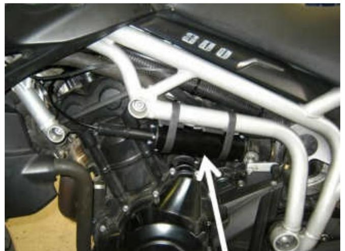
On the Tiger 800 XC, the **Electric Throttle Servo (2)** must be fitted to the lower frame tube on the rear sub-frame using hose clamps to attach it to the frame. The positions of the servo along the frame tube can be selected. The servo can be mounted directly above the passenger foot rests (photo left below) or further back along the tube (photo right below).
