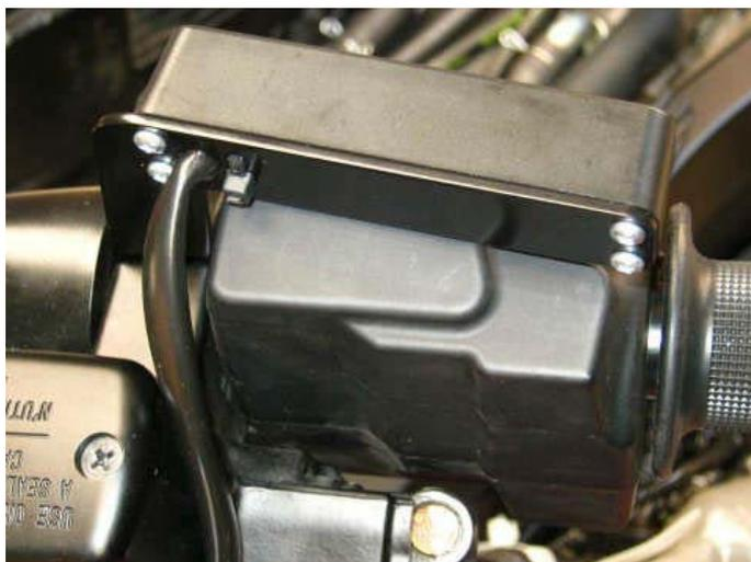
An **OPTIONAL** mounting arrangement is available for the **Control Switch (6)**. This arrangement places the control switch in a similar position, but it is screwed to the removable top cap of the bike's left side switch block. The bracket is cut to 'fit' the top of the bike's switch block. This requires that 2 holes are drilled in the cap. This is still fairly easy to install, but requires partial disassembly of the bikes left hand switch block to fit it.
