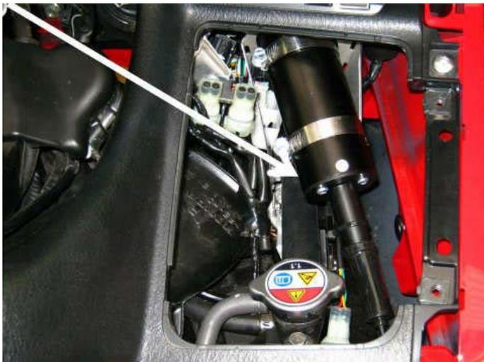
A **lost motion device (4)** is fitted to the end of the throttle spindle on the throttle body. This device is fitted to allow safe operation of the cruise control and twist grip without risk of the servo cable twisting or jamming.
