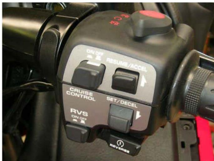
We can supply information to 'build' a suitable circuit to turn the RVS button into a Hazard Light button, but this does require an installer with some electrical knowledge. Re-labelling the button is another small issue, but not a critical one. We are not in a position to provide the necessary components to do this.
