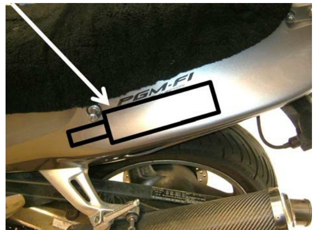
The Electric Throttle Servo (2) is mounted on the left side of the bike, under the seat fairing panel. The photo below shows the bike with the seat fairing fitted above with the servo mounted to the frame without the panel fitted. A cable connects it to the CIU (3).
