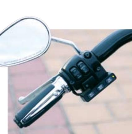
**11** A close up of the controls that are lit for night time operation. The switches selected for cruise control operation have been chosen as they are large enough to be readily activated by gloved fingers.
