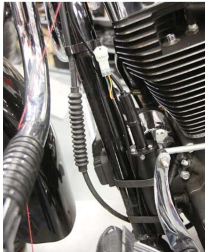
**1** Craig begins by fitting the electric throttle servo to the left side front down tube using the two covered hose clamps supplied in the kit. The servo cable which can be seen at the top he then routes through the frame to the bike's throttle body and connects it to the existing cable bracket and then adjusts the cable free play to the supplied specifications.
