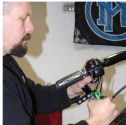
**2** Craig now installs the control switch block below the left handlebar switch block and then routes the switch wiring through the handlebars.
