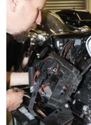
**9** In the process of connecting the cruise control wiring Craig takes the opportunity to tidy up some of the wiring from previous electrical installations on the bike including an amplifier, heated grips and a couple of other aftermarket components.
