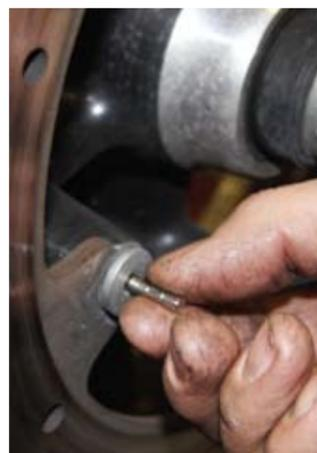
**4** And then places each of the supplied magnets into the heads of the front disc brake mounting bolts.
