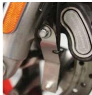
**3** He now positions the speed sensor bracket using the caliper bolt.
