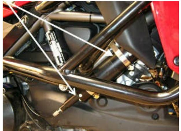
The **CIU (3)** is located on the left side of the engine. A new **cable (4)** connects the CIU to the throttle bodies.
